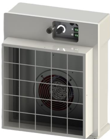
Suction box for HEPA filtration HEPA H14 filter allowing a maximum 0.005% of 0.1 micron particles to pass Nominal flow : 150 m 3 /h Dimensions : 420 x 341 x 146 mm
