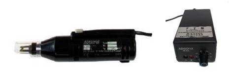
Electric stripping machine for varnished wires, the abisofix consists of a motor group and a stripping head. The stripping head is equipped with 3 hard metal blades. The blades are closed thanks to the rotation. The speed is regulated by transformer and the pressure force of the blades is adjusted to each material thickness.
