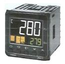
To increase the case temperature, press the right button until the green indicator shows the desired set point.
