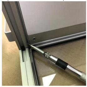
Insert the top profile of the cab onto the side panel, secure it with the screw.
