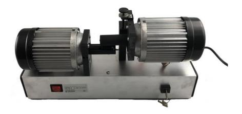
BTM 2 is a table-mounted stripping device for flat enamelled and round copper wire, the range of 0.2 to 6 mm can be stripped. It is possible to modify the axis of the machine to use brushes of different diameter (22mm, 30mm or 40mm).
