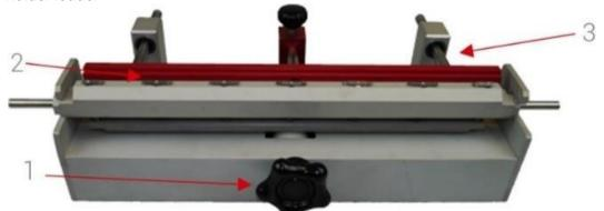
This device was studied to facilitate the loading and the unloading of components in particular those concerning the hybrid components, Flatpacks, Quad packs etc. A button (1) activates a cam and raises the springs (2) to let the components pass. In addition, this device makes it possible, by means of its adjustable stop (3), to wedge the component on the bar in a predetermined position, for example by centering them so as to be able to tin the 2 sides by turning it over.
