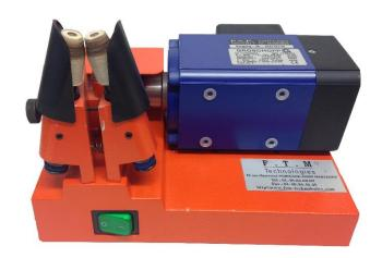
Designed for wires from  $\emptyset$  0.04 to  $\emptyset$  0.3 mm. The spacing of the brushes is adjustable by a knurled screw.
