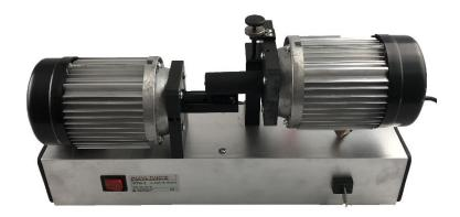
BTM 2 is a table-mounted stripping device for flat enamelled and round copper wire, the range of 0.2 to 6 mm can be stripped. Brush diameter according to the machine version 22 mm.
