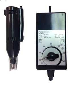
Electric stripping machine for varnished wires, the abisofix consists of a motor group and a stripping head. The stripping head is equipped with 3 hard metal blades. The blades are closed thanks to the rotation. The speed is regulated by transformer and the pressure force of the blades is adjusted to each material thickness.
