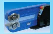
Motorized machine suitable to separate pre-assembled Electronic Board. Precise, reliable and safe. The PCB is manually fed between the lower and upper blades using the scoring as reference. By pushing the board horizontally, the blade rotation starts offering a sharp and accurate cut. The blade height is adjustable depending on the thickness of the PCB.
