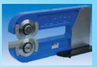
Manual machine suitable to separate pre-assembled Electronic Board. Precise, reliable and safe. The PCB is manually fed between the lower and upper blades using the scoring as reference. By pushing the board horizontally, the blade rotation starts offering a sharp and accurate cut. The blade height is adjustable depending on the thickness of the PCB. Upper and lower blades are also available titanium pleated version
