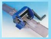
The model SEF 1 is designed for separating wires of flat cables. Two different pitches of separation can be supplied: 1,27 mm (the wires are individually separated Code 73.0L01) or 2,54 mm (the wires are separated by couples Code 73.0L02). This version is a "bench" manual machine suitable for separating edges of flat cables having maximum width of **XX**mm.
