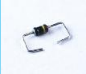
SP36.03 AXIAL LOOSE COMPONENTS FORMING
