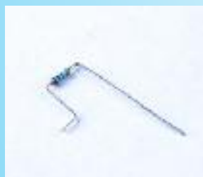
48.0L02.06 CUT AND "SEAGULL WINGS" FORM
