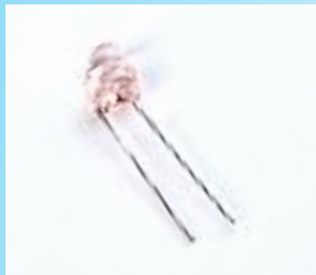
SP38.02 LOOSE L.E.D. CUT AND RIGHT BEND
