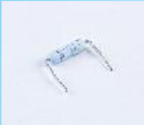
48.0L01 CUT BEND AND FLATTEN LEADS
