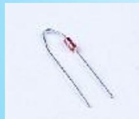
SP22.21 CUT AND BEND FOR VERTICAL MOUNT
