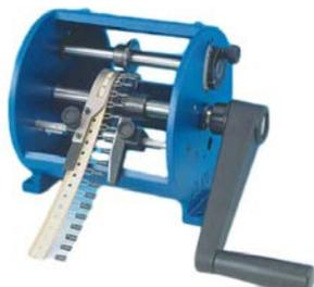
Machine cambrage composant radial
