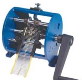
Machine cambrage composant axial
