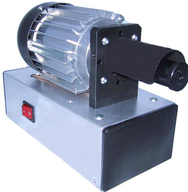
The Abfräsfix is a electrical stripping machine for varnished wires. The wire is pushed into the rotating stripping-head up to the lengthstop. Thereby five blades are milling the varnish away. Strippinglength and -diameter are steplessly variable. For heavy workparts it is possible to use a flexible shaft. The machine will be delivered with blades of tool steel. For very strong varnish we can deliver blades of hard metall.
