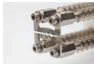
CCT: Thermal knife (braid cutter, frets, etc.)
