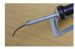
Optional: To increase the accuracy and quality of your work, this iron can be connected to the power regulator RP500 which allows operation over a wide range of temperatures from 20 to 350°C max.
